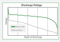
Discover AES batteries have a flat and stable discharge curve, which can not be accurately monitored by a voltage based SOC indicator. For accurate fuel gage and SOC an AES compatible Battery Discharge Indicator is necessary.
