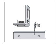
\*When used in conjunction with the S-5-PV Kit, an extra nut is necessary to secure ProteaBracket's slotted L-flange to the universal PV stud and mounting disk.
